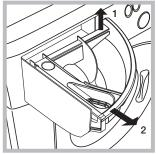
Remove the dispenser by raising it and pulling it out (see figure). Wash it under running water; this operation
